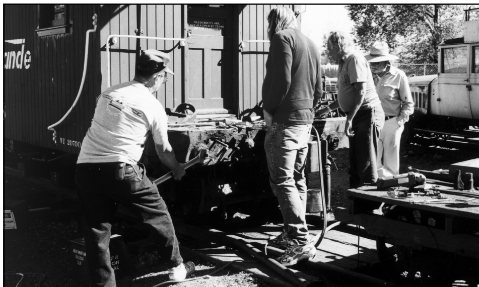
From left; Phil Scholl takes his turn loosening a truss rod nut while Matt Toman heats the next nut. Bob Tully completes the removal of an nut while Russ Stuska assists with the tools. – Photo © Steve Mason
